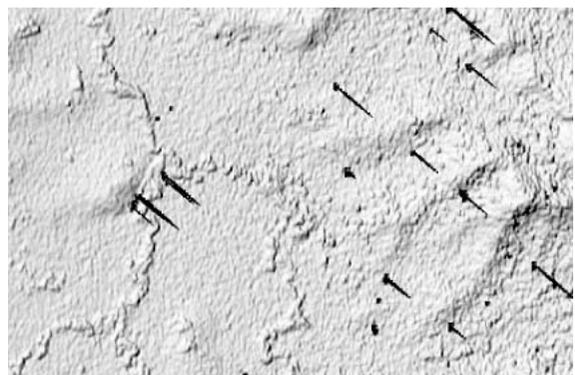
Fig 3. Shaded relief view of a 10-m-resolution DEM obtained from airborne SAR in an area with low relief.
