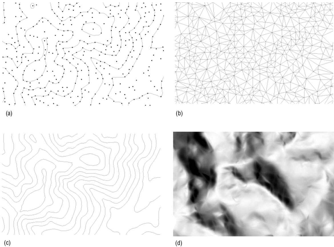
**Fig 4.** Interpolation of surface-specific elevation data using triangulation: (a) surface-specific points overlaid with the contour data from Figure 2; (b) TIN derived from the surface-specific points; (c) contours interpolated from the TIN; and (d) shaded relief view of the surface interpolated from the TIN.
